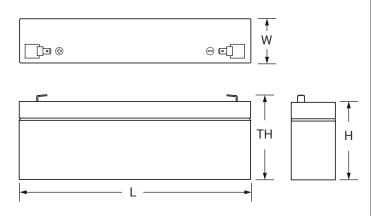
L: 7.01 (178) W: 1.36 (34.5) H: 2.38 (60.5) TH: 2.60 (66) Tolerances are +/- 0.04 in. (+/- 1mm) and +/- 0.08 in. (+/- 2mm) for height dimensions. All data subject to change without notice.
