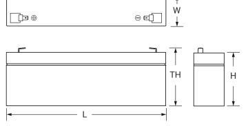
Tolerances are +/- 0.04 in. (+/- 1mm) and +/- 0.08 in. (+/- 2mm) for height dimensions. All data subject to change without notice.
