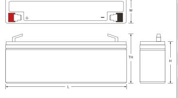
**L:** 7.01 (178) **W:** 1.38 (35) **H**: 2.36 (60) **TH:** 2.60 (66) Tolerances are +/- 0.04 in. (+/- 1mm) and +/- 0.08 in. (+/- 2mm) for height dimensions.
