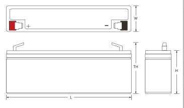
L: 7.01 (178) W: 1.38 (35) H: 2.36 (60) TH: 2.60 (66) Tolerances are +/- 0.04 in. (+/- 1mm) and +/- 0.08 in. (+/- 2mm) for height dimensions. All data subject to change without notice.
