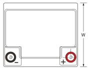
7.76 (197) 1: W: 6.50 (165) **H:** 6.69 (170) **TH:** 6.69 (170) Tolerances are +/- 0.04 in. (+/- 1mm) and +/- 0.08 in. (+/- 2mm) for height dimensions. All data subject to change without notice.
