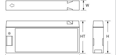
**L**: 7.17 (182) **W**: 0.94 (24) **H**: 2.40 (61) **HT**: 2.40 (61) Tolerances are +/- 0.04 in. (+/- 1mm) and +/- 0.08 in. (+/- 2mm) for height dimensions.
