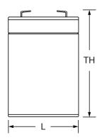
L: 2.76 (70) W: 1.85 (47) 3.94 (100) TH: 4.17 (106) Tolerances are +/- 0.04 in. (+/- 1mm) and +/- 0.08 in. (+/- 2mm) for height dimensions. All data subject to change without notice
