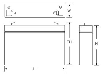
L: 5.91 (150) **W:** 1.34 (34) **H:** 3.70 (94) **TH:** 3.94 (100) Tolerances are +/- 0.04 in. (+/- 1mm) and +/- 0.08 in. (+/- 2mm) for height dimensions. All data subject to change without notice.
